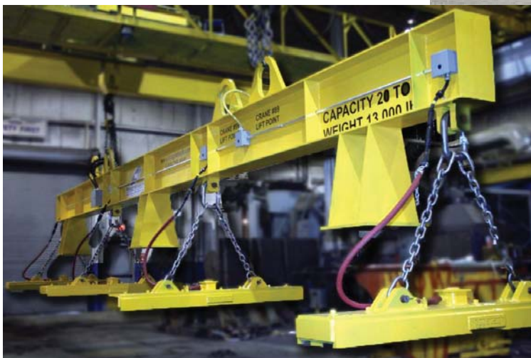
Custom spreader beam and magnets with PowerPro generator fitted to a Taylor Equipment loader.
