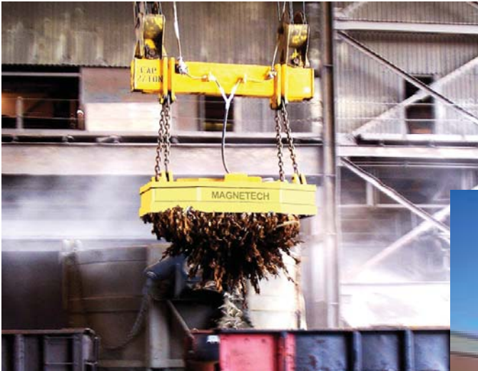
120" x 85" Scrap Magnet Custom Engineered for Magnetech Customer Increased Lifting Capacity of Previously Used Dual Magnets by 20%.
