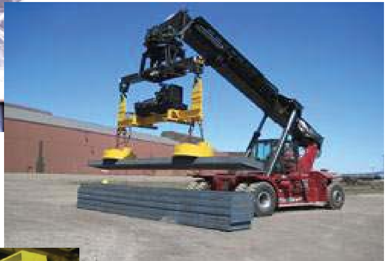
Custom spreader beam and magnets with PowerPro generator fitted to a Taylor Equipment loader.
