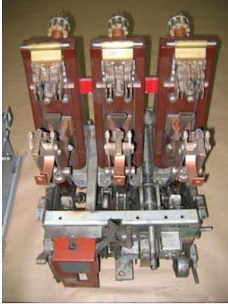
Circuit breaker repaired and retrofitted for Cinergy, before and after.
