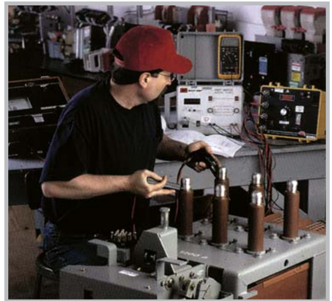
All levels of service include contact resistance testing.
